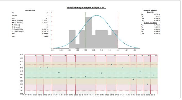
In the screenshot above, the ei<sup>3</sup> system summarizes measurements taken in the continuous manufacturing process, visualizing the spread of the measurement variable across the desired value. Cut-off lines on either side visualize allowable bands. Operators immediately see if the plant is operating at excess waste, i.e., measurements falling outside those bands.
