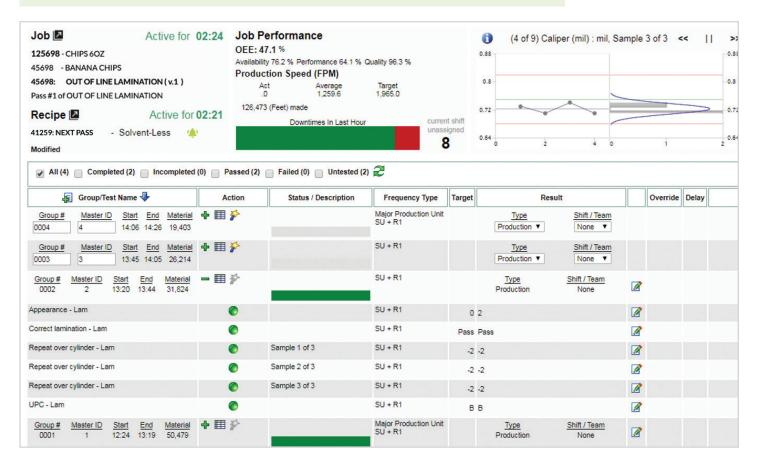
In the screen show above, the ei<sup>3</sup> system visualizes continuous measurements taken on an operating line; immediately giving operators feedback on results, including "Pass" and "Fail".
